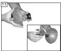
Install canopy and yoke cover over the down-rod.
